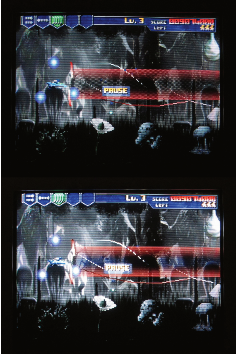
Figure 15: Mesh effect on a CRT TV connected through an RGB SCART cable (top) and a composite cable (bottom).
