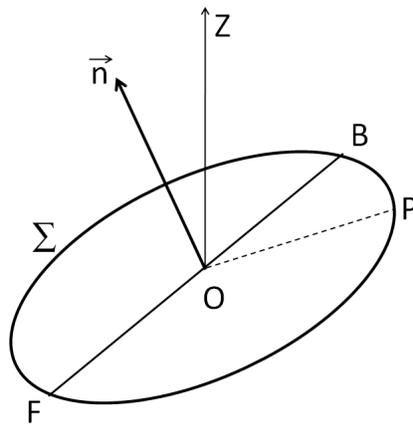
**Figure 7.** Vertical axis OZ associated with the artificial horizon provided by an aircraft's navigation instrument, and the vertical perceived by the pilot (vector  $\vec{n}$ ) associated with the plane of the device,  $\Sigma$
