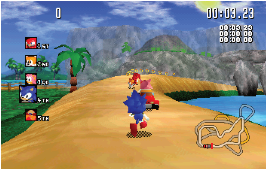
Figure 17a: Objects near the horizon are drawn half-transparent with a gradient based on the distance from the camera (fade-in effect).
