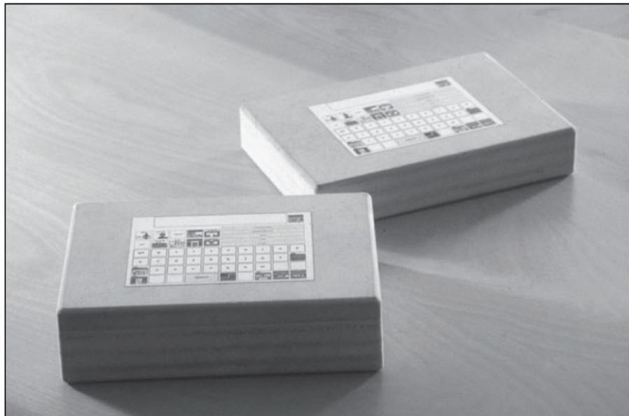
**Figure 5.4** Block-level prototypes that are precursors to a hand-held augmentative communications device. (Reprinted with permission of Daedalus)
