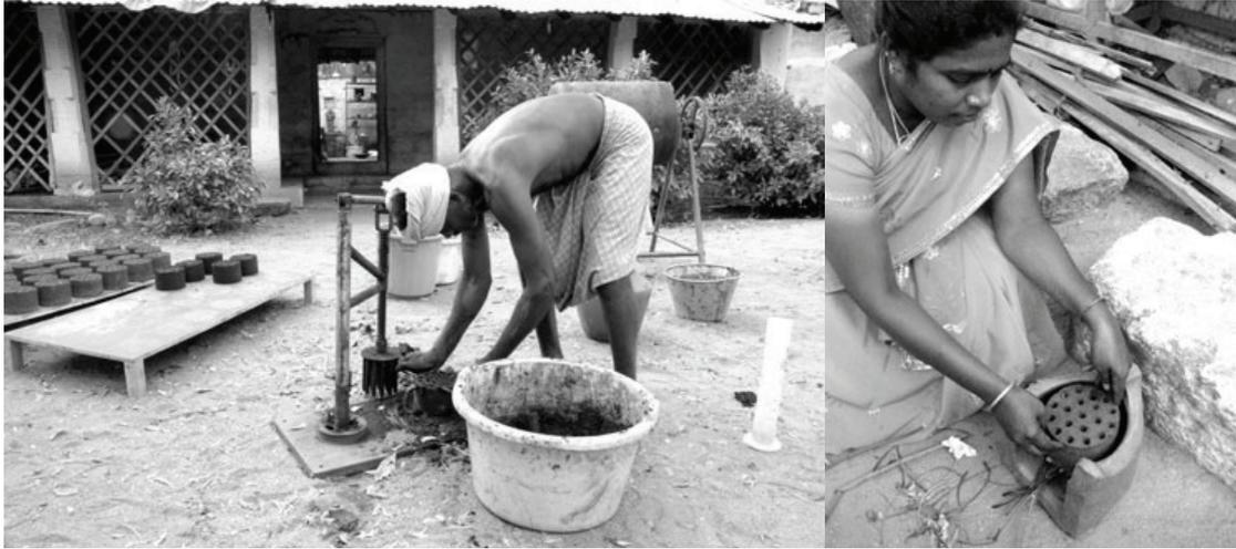
**Figure 10.5** Charcoal briquettes made locally in India with the Design Impact briquette maker. (With permission of Design Impact)
