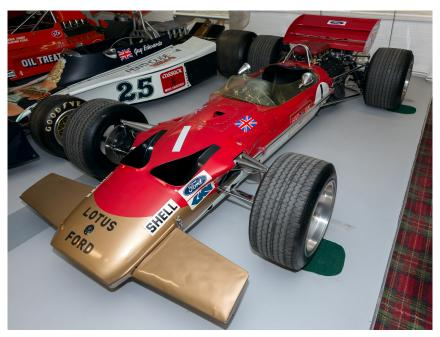
Figure 1. The Louts 49B features front and rear wings. (Credit: Morio)
