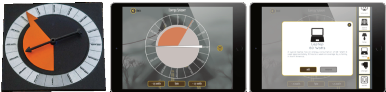
Figure 2. a) Close-up of the power spinner. The orange area is variable & conveys current energy usage based on game state (b) Power spinner on an iPad app (on the whole-home extension of Energy Monsters) that also takes input from household infrastructure to affect game state. (c) Energy consumption data shown on the app.
