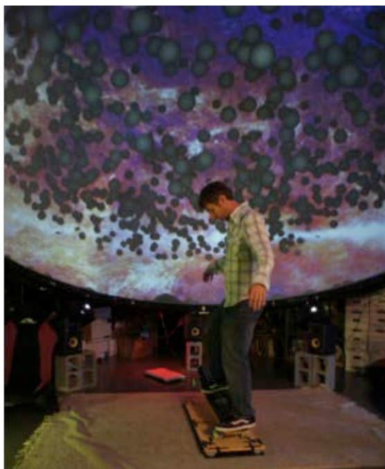
Figure 1: Similar to a small planetarium, our 15-ft diameter dome can accommodate 12 learners. Six projectors powered by one Mac Pro allow for multi-user interactivity. Here, DomeStroids is controlled with a WiiMote and pressure sensors in a skateboard interface.
